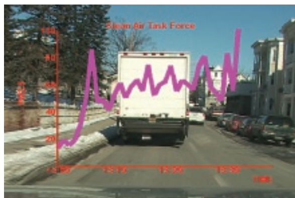
Solutions that work: CATF's installation of a diesel particle filter on a box truck dramatically reduced fine particles ( PM_{2.5} ) near the tailpipe from 5,000 \mu\text{g}/\text{m}^3 to 25 \mu\text{g}/\text{m}^3 . As a result, fine particles from the truck barely registered in the car following behind. To view videos, go to www.catf.us/goto/noescape/
