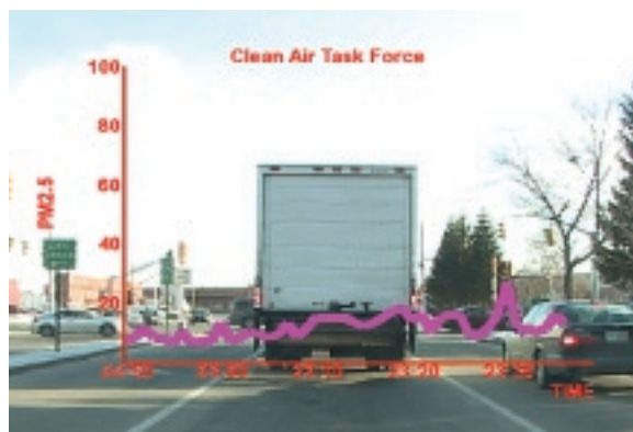
Solutions that work: CATF's installation of a diesel particle filter on a box truck dramatically reduced fine particles ( PM_{2.5} ) near the tailpipe from 5,000 \mu\text{g}/\text{m}^3 to 25 \mu\text{g}/\text{m}^3 . As a result, fine particles from the truck barely registered in the car following behind. To view videos, go to www.catf.us/goto/noescape/
