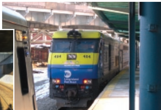
When pulled by a locomotive (left), pollution from the engine invades the coaches behind. When the train is pushed, the pollution plume trails behind leaving in-coach levels low (right).
